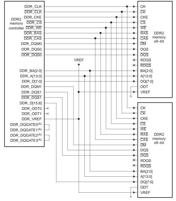
Figure 19. Connecting to Two 8-Bit DDR2 SDRAM Devices
